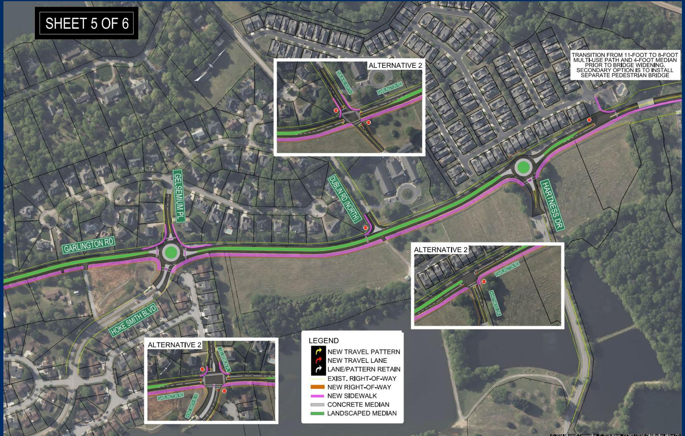
TRANSITION FROM 11-FOOT TO 8-FOOT MULTI-USE PATH AND 4-FOOT MEDIAN PRIOR TO BRIDGE WIDENING. SECONDARY OPTION IS TO INSTALL SEPARATE PEDESTRIAN BRIDGE
