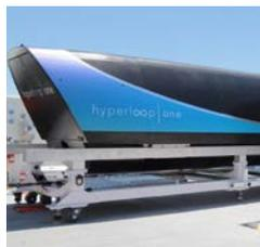
Currently in development as an experimental transportation method, the Hyperloop connects two destinations with a sealed tube that transports passenger pods at high speeds. A hyperloop network would connect regional destinations similar to a rail network.
